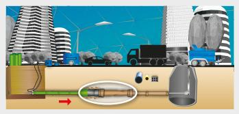
Trenchless renewal in the existing pipe path. Installation of the new pipes with identical or larger nominal diameters.
