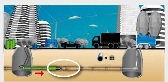
Short or long pipe relining of concrete or stoneware pipes. The new pipe fits tightly inside the old pipe.
