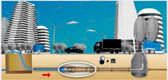
Partial damage is expanded dynamically and a new pipe is pulled in simultaneously.
