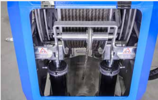
Double cylinder drive - powerful and even
