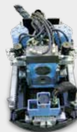
GRUNDOPIT S for bores out of a manhole
