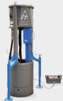
GRUNDOPIT K for bores out of a circular bore hole (Keyhole)
